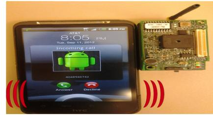
Fig. 8. Incoming Call Experiment (Left: Android device; Right: MTS310CB with accelerometers)
