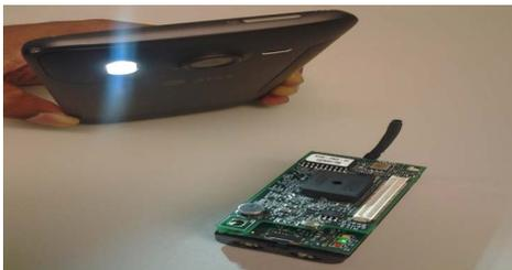
Fig. 4. Morse Code Experiment (Left: Android device; Right: MTS310CB with light sensors)
